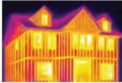
Thermal energy is lost through uninsulated framing. This is a graphic depiction of heat loss in a typical home. Yellow areas indicate the greatest energy loss.
